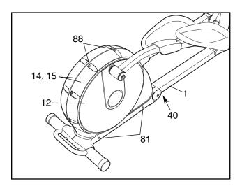
Adjust the position of the Side Shields (14, 15) until the Discs (12) no longer rub against them, and then tighten the Bolt Sets (88) and the #8 x 1/2" Screws (81).
